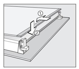
Finally replace the black printed inner pane. The print should face the middle pane.
